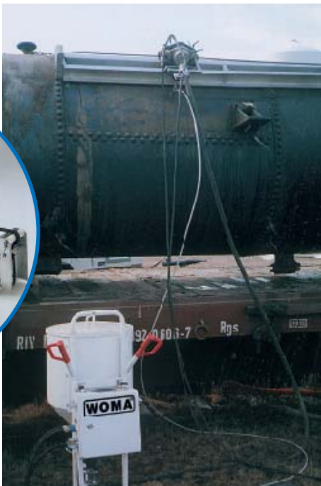
Pneumatically driven water jetting tool type Top Cutter for steel and rebar structures
