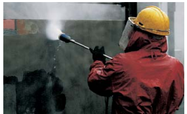
High-pressure gun with self propelling rotating nozzle carrier head type TD 2100 for derusting of steel panels
